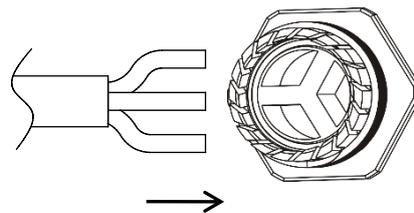
b. Insert the cable end into the seal.
