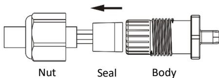
d. Rotate the nut with 3.3N·m until the latching mechanism meets the base.
