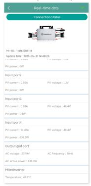
Note: If the microinverter signal is so weak that the real-time data are not updated, move the DTU closer to the microinverter.
