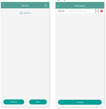
6. Scan or manually input the microinverter ID. Press "Finish" when all microinverter IDs have been input.
